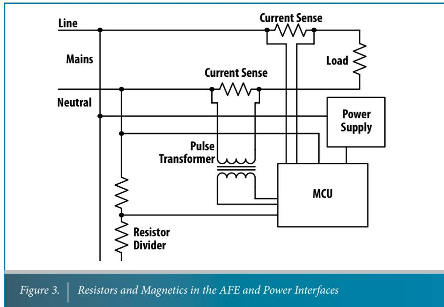
Figure 3. | Resistors and Magnetics in the AFE and Power Interfaces
