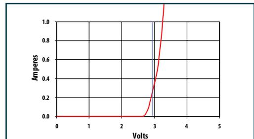
Figure 4. Typical V-I Curve for an LED
