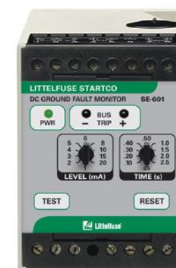
Figure 2. The SE-601 DC Ground-Fault Monitor provides sensitive, fast ground-fault protection with nuisance tripping. Ground-fault current is sensed using an SE-GRM Series Ground-Reference Module—a resistor network that limits ground-fault current to 25 mA. The SE-GRM allows an SE-601 to be connected to systems up to 1200 Vdc and potentially higher.
